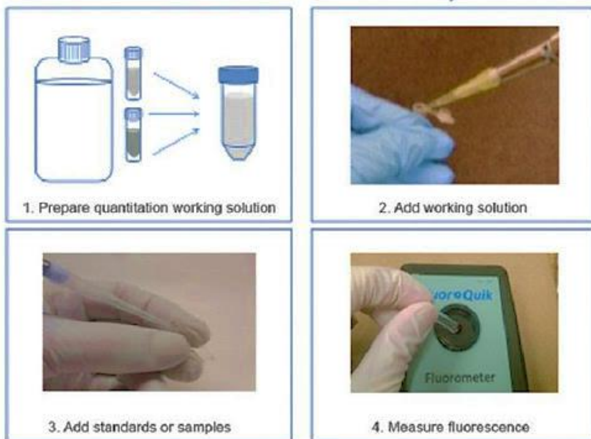
Figure 75- Example of a fluorescence detection methods used to quantify DNA concentration following extraction. The dyes can be used to easily quantify a large number of dsDNA samples (AmiScience 2018).
