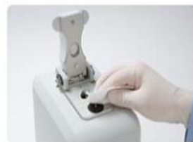
Figure 76- A NanoDrop machine is typically used to assess the purity and concentration of extracted nucleic acid. Very small quantities of a sample (0.5-2 \mu L) are added to the NanoDrop pedestal as shown above, rapidly measured by spectrophotometry and then wiped clean before adding the next sample (ThermoFisher 2021).
